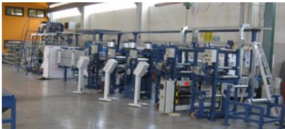
Fig. 2. Technological complex of impregnation for preregs purchased for BACO Prospects for the use of preregs in the manufacture of other parts.
