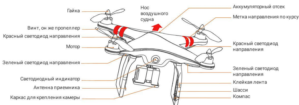
Figure 1 Design of an unmanned aerial vehicle
